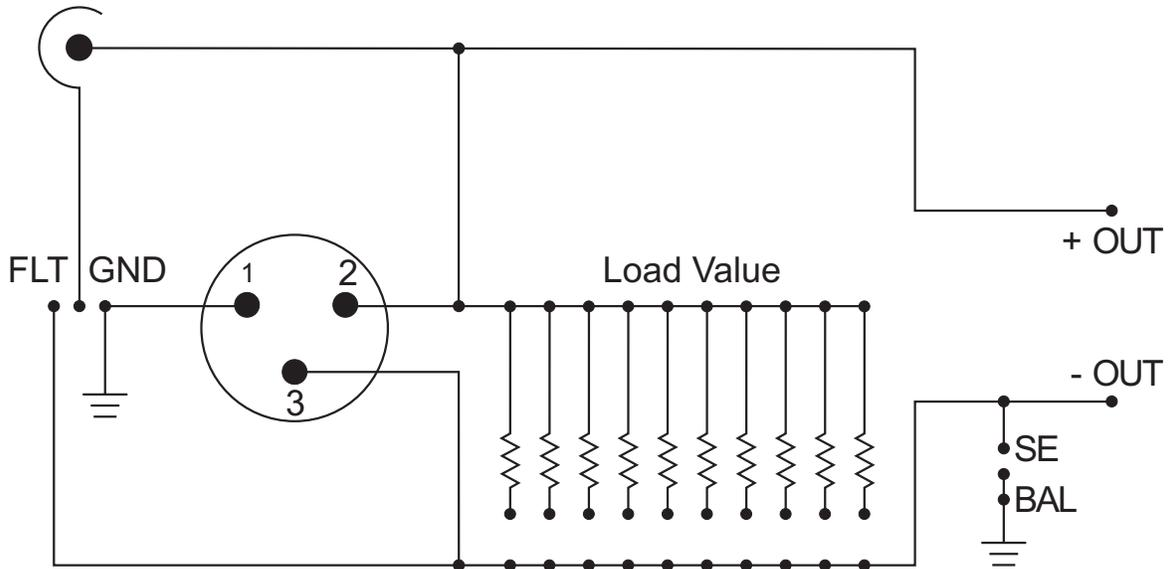
Aux Input board phono section block diagram
